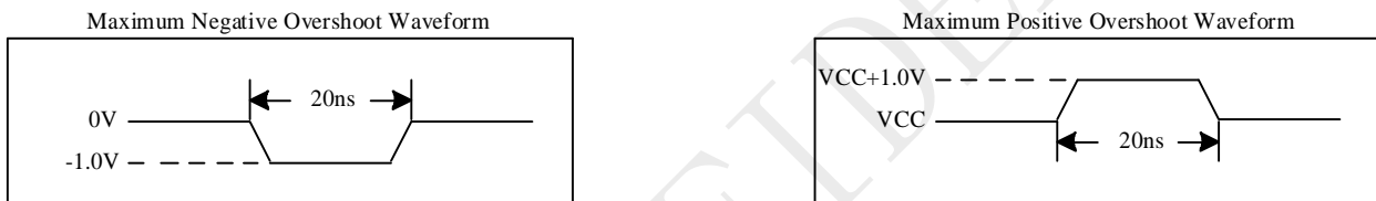
Figure 5-2 Input Test Waveforms and Measurement Level
